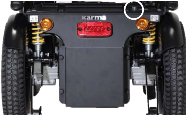
Circuit breaker location
