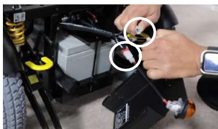
Step 7: Untighten these 4 knobs on the both sides to take off back-rear cover.
