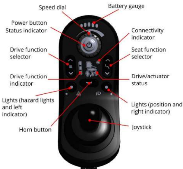
Control Panel with No Tilt & Lighting System
