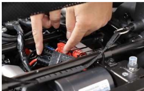
Step 6: After the top-back cover is off, you will see two power connector. One is red and one is black. Disconnect the power cables.
