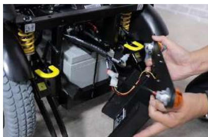
Step 7: Untighten these 4 knobs on the both sides to take off back-rear cover.
