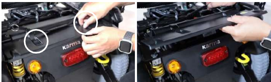
Step 5: Untighten these 2 knob to take off the top-back cover.
