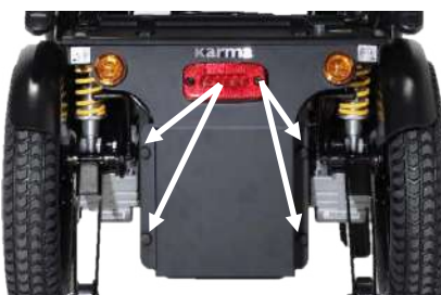
Step 7: Untighten these 4 knobs on the both sides to take off back-rear cover.
